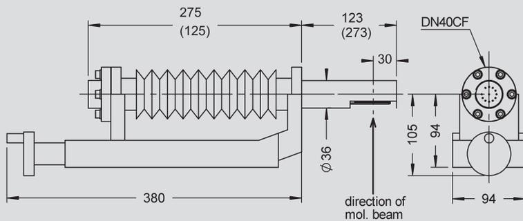
Schematic drawing of the Beam Flux Monitor BFM
