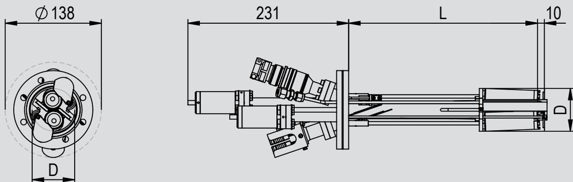
Schematic drawing of the Dual Doping Source DDS
