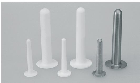
Different ceramic and metal crucibles (1.5 and 10 cm<sup>3</sup>) for HTEZ
