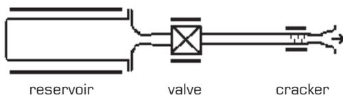
Schematic drawing of the VCCS all-PBN assembly of crucible, valve and cracker, surrounded by three independent heaters
