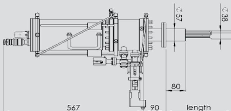
Schematic drawing of the Valved Corrosive Cracker Source VCCS
