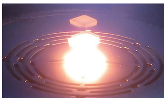
CO2 laser substrate heating: Many oxide substrates absorb CO2 laser light strongly, allowing substrate heating up to more than 1400°C. An additional backside metal coating is not necessary. (Courtesy of Prof. J. Mannhart, MPI-FKF Stuttgart)
