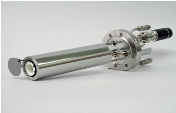
Organic Effusion cell OEZ 63-35-33-S: OEZ source with 35 cm 3 crucible, mounted on a DN63CF (O.D. 4.5") flange, with integrated water cooling and rotary shutter
