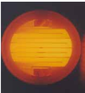
Front view of hot carbon filament (operation after removal of orifice plate)
