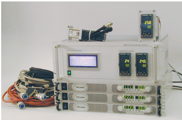
Additional equipment for the VCCS (motorized valve control unit MVCU with temperature controllers, power supplies and cables)
