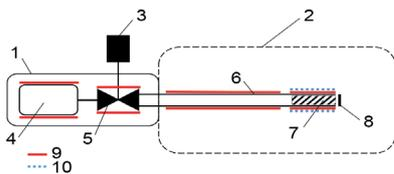
Schematic of VSS. 1 case, 2 vacuum chamber, 3 stepper motor for valve regulation; 4 material reservoir, 5 valve, 6 PBN injector tube, 7 cracker insert, 8 shutter, 9 electrical heater, 10 water cooling
